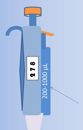
This is a <u>Micropipette</u> it is used to accurately transfer small quantities of liquid.
